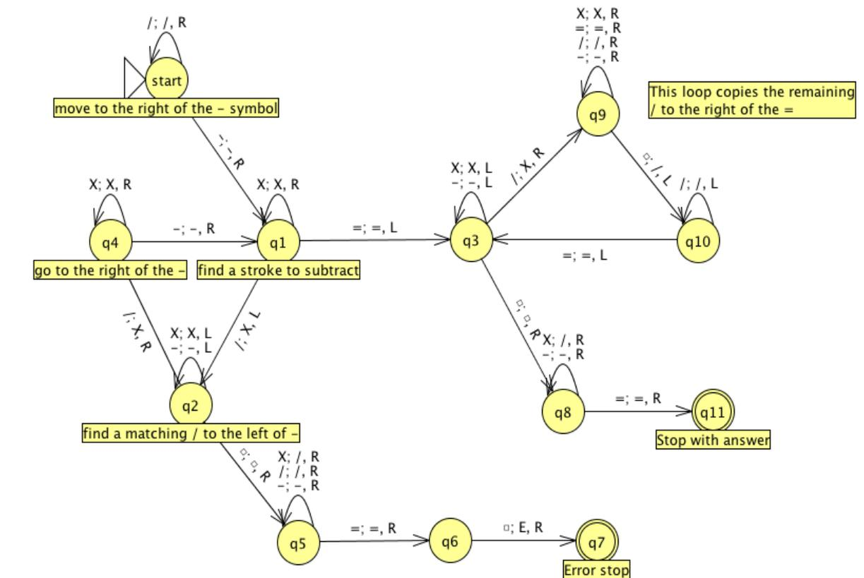
The approach show below performs subtraction by first moving to the “-” symbol on the tape, finds a stroke to the right of the “-”, then looks for a stroke to the right and marks it, state  $q_1$ . State  $q_2$  find a stroke to the left of the “-”. The  $q_1$ - $q_2$ - $q_4$  loop continues pairing the strokes until it finds the “=” symbol in  $q_1$ , or does not find a match in  $q_2$ .
